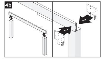
4b. Attach beam to post using NCS front and back beam brackets with required fasteners. See Required Fasteners chart on page 6, column A, for approved metal-to-metal fasteners for attaching brackets to beam.
