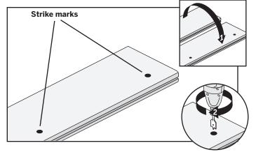
Flip board over so that bottom of board faces up and shows strike marks from the screws. Using a paddle drill bit, carefully drill holes to the depth of the fastener heads in the joist. Flip board over so that drilled holes
