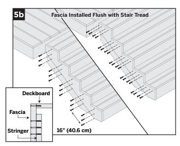
5b. Fasten fascia boards to deck boards from the side as shown. Three fasteners are required every 16" (40.6 cm) for fascia into stringer and two are required to attach fascia into each deck board. See Required Fasteners chart on page 6, column B.
