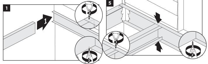
1. Slide the joist within the flanges of the track and rest the outer end on the support post or beam. Fasten joist to track using required fasteners. See Required Fasteners chart on page 6, column A. Fasten through the track flange into the joist on top and bottom.
