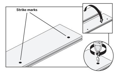
Flip board over so that bottom of board faces up and shows strike marks from the screws. Using a paddle drill bit, carefully drill holes to the depth of the fastener heads in the joist. Flip board over so that drilled holes fit over joist fasteners, and fasten board per instructions.
