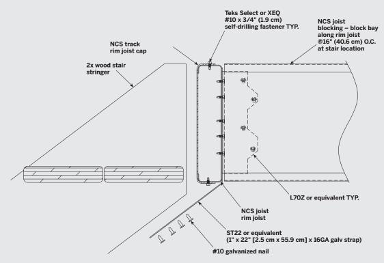
WOOD STAIR ATTACHMENT TO RIM JOIST CAP
