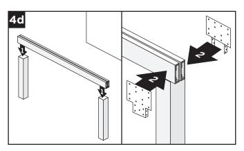
4d. Attach beam to post using NCS front and back beam brackets and required fasteners. See Required Fasteners chart on page 6, column A, for approved metal-to-metal fasteners for attaching brackets to beam.
