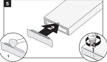
5. Secure cap with exterior grade metal adhesive and/or  $\#10 \times 3/4$ " (1.9 cm) self-tapping screws.
